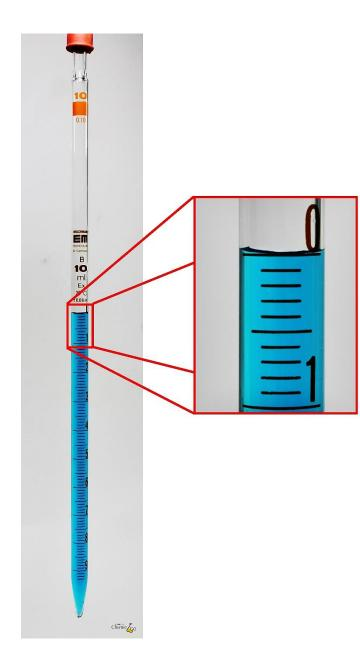
When using a pipette, the solution is taken up until the 0 (zero) mark (lower edge of the meniscus).
