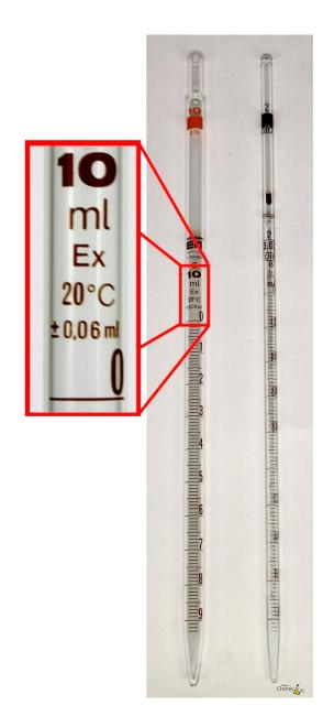
Typically, all volumetric instruments are provided with details regarding accuracy and application.
