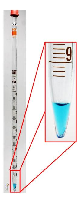
The measured volume results from the difference after liquid release.
